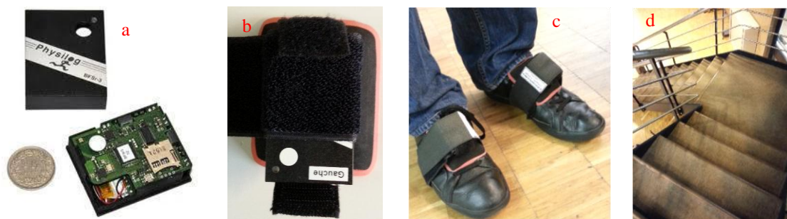
Figure 1-a) Physilog® with data logger, b) Physilog® inserted in a strap, c) Sensors attached to participant's feet, d) Staircase used for monitoring stair descent and ascent. Note the level platform in the middle of the stairs.
